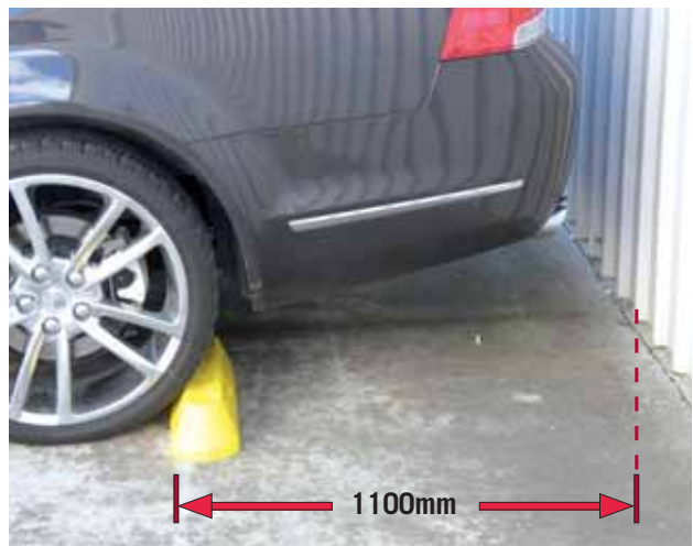
Rear into a high kerb or wall.
